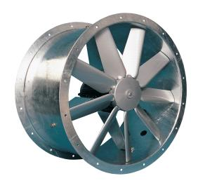
The Fläkt Woods impellers are all high pressure die cast to offer thin aerofoil sections for low generation of noise. Every cast aluminium component is X-ray examined using Real Time Radiography inspection prior to assembly. The maximum pitch angles shown are based on speed control by frequency inverter. This range is available in Form B only (air entering the impeller first).
